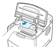
If the jammed paper is not visible or there is resistance when you pull the paper, go to "In the Paper Exit Area" on page 7.12.
